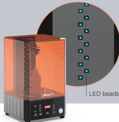
DOUBLE-ROW AND DOUBLE-BAND UV LAMP BEADS
