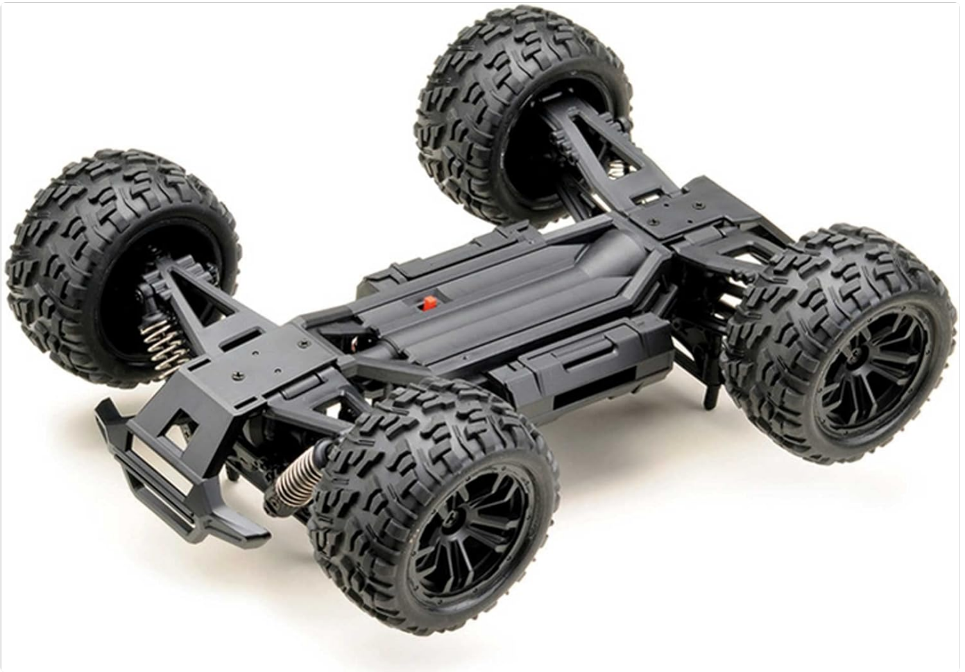
Image 4.2.1: Underside view of the Absima RC truck chassis. The battery compartment is visible in the center, designed for easy access.
