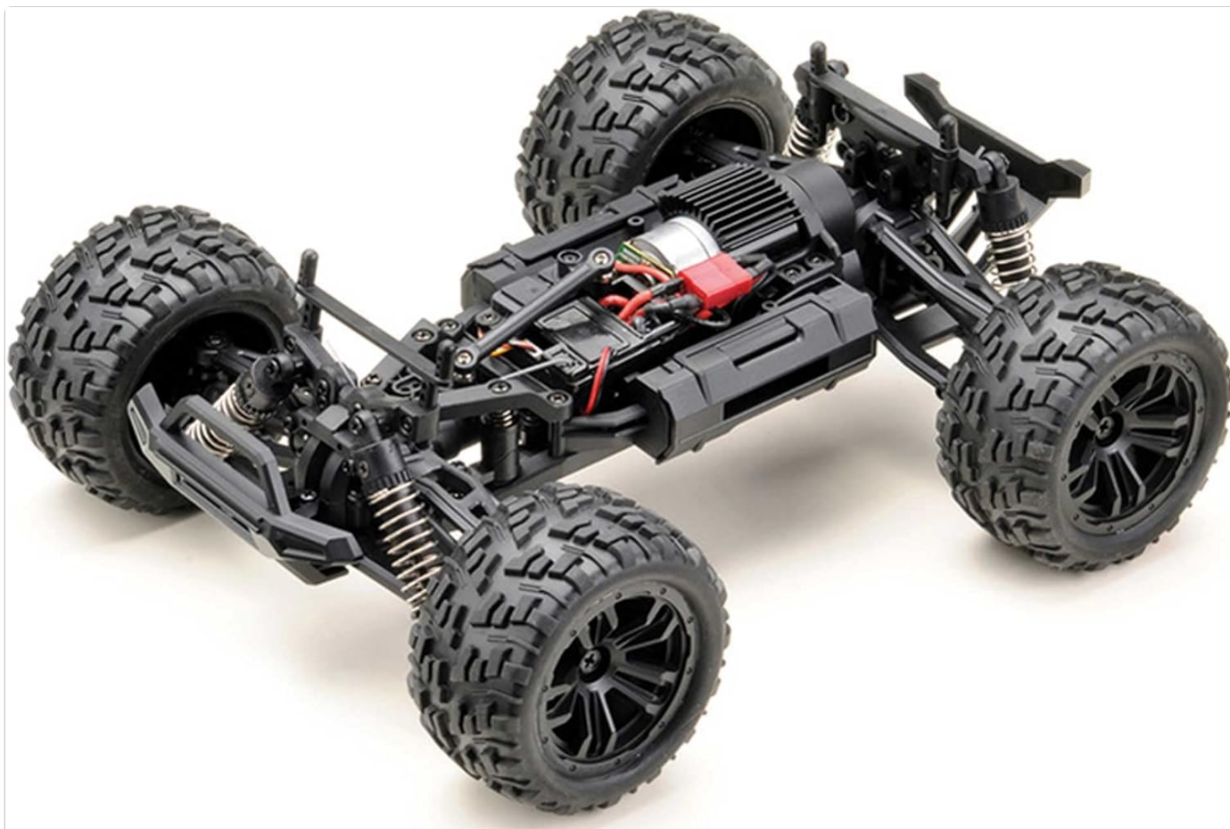
Image 5.1.1: Top-down view of the Absima RC truck chassis with the body removed, showing the motor, electronics, and suspension components. This view highlights the internal layout for maintenance and understanding controls.
