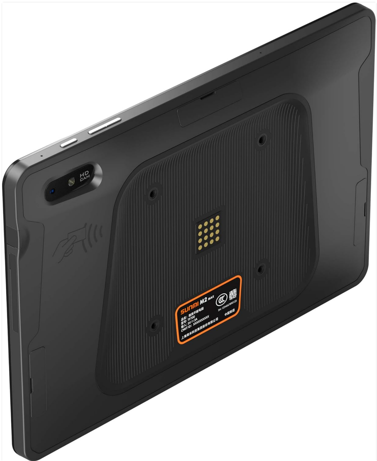
Figure 2: Rear view of the SUNMI M2 MAX, highlighting the camera, pogo pin charging interface, and the location of the SIM/MicroSD card slot.
