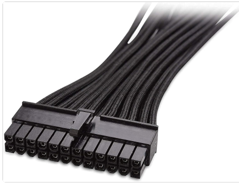
Image: Close-up of the male end of the ATX 24-pin cable.
