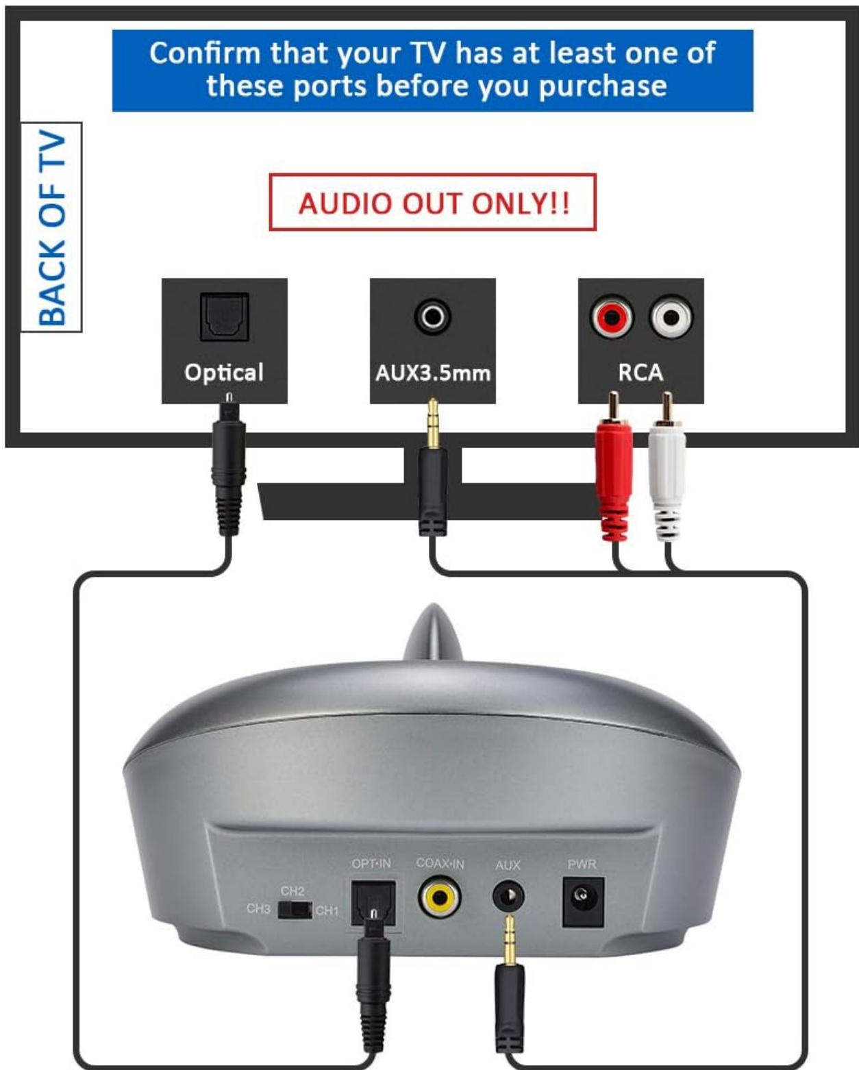
Image 4.1: Connecting the transmitter to various TV audio output ports.
