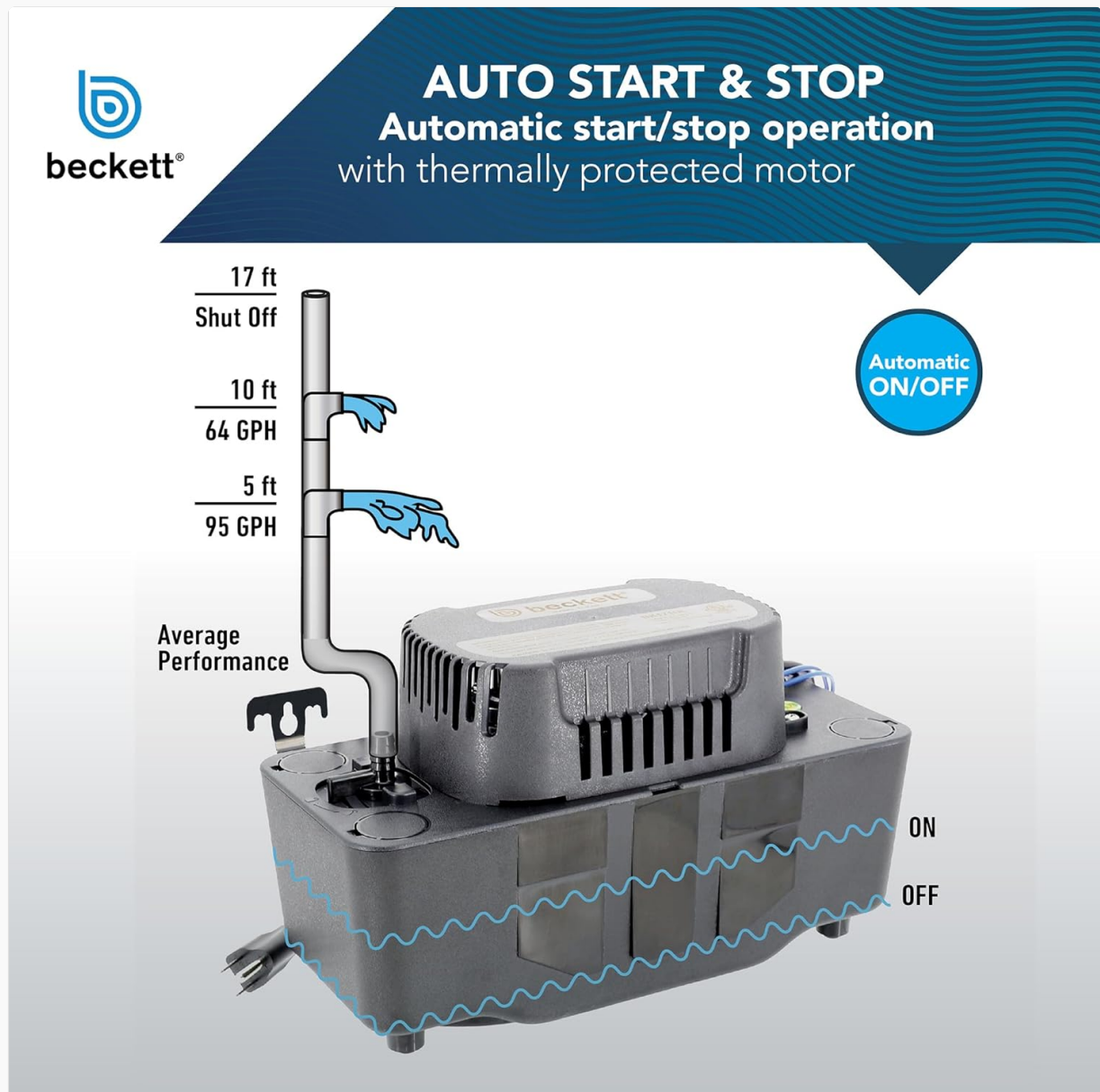
Image 5.1: Diagram illustrating automatic ON/OFF operation and average performance at various lift heights (e.g., 95 GPH at 5 ft lift, 64 GPH at 10 ft lift, 17 ft shut-off).
