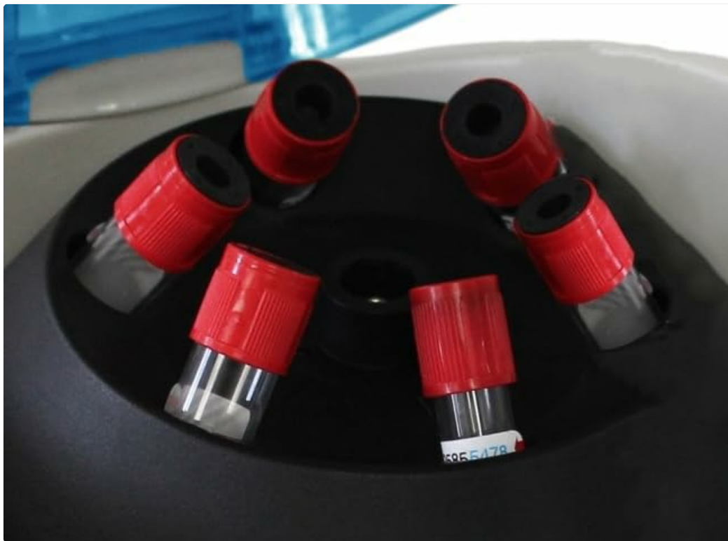
Figure 3: The rotor of the SCI-506 centrifuge, designed to hold 6 tubes with adapters.
