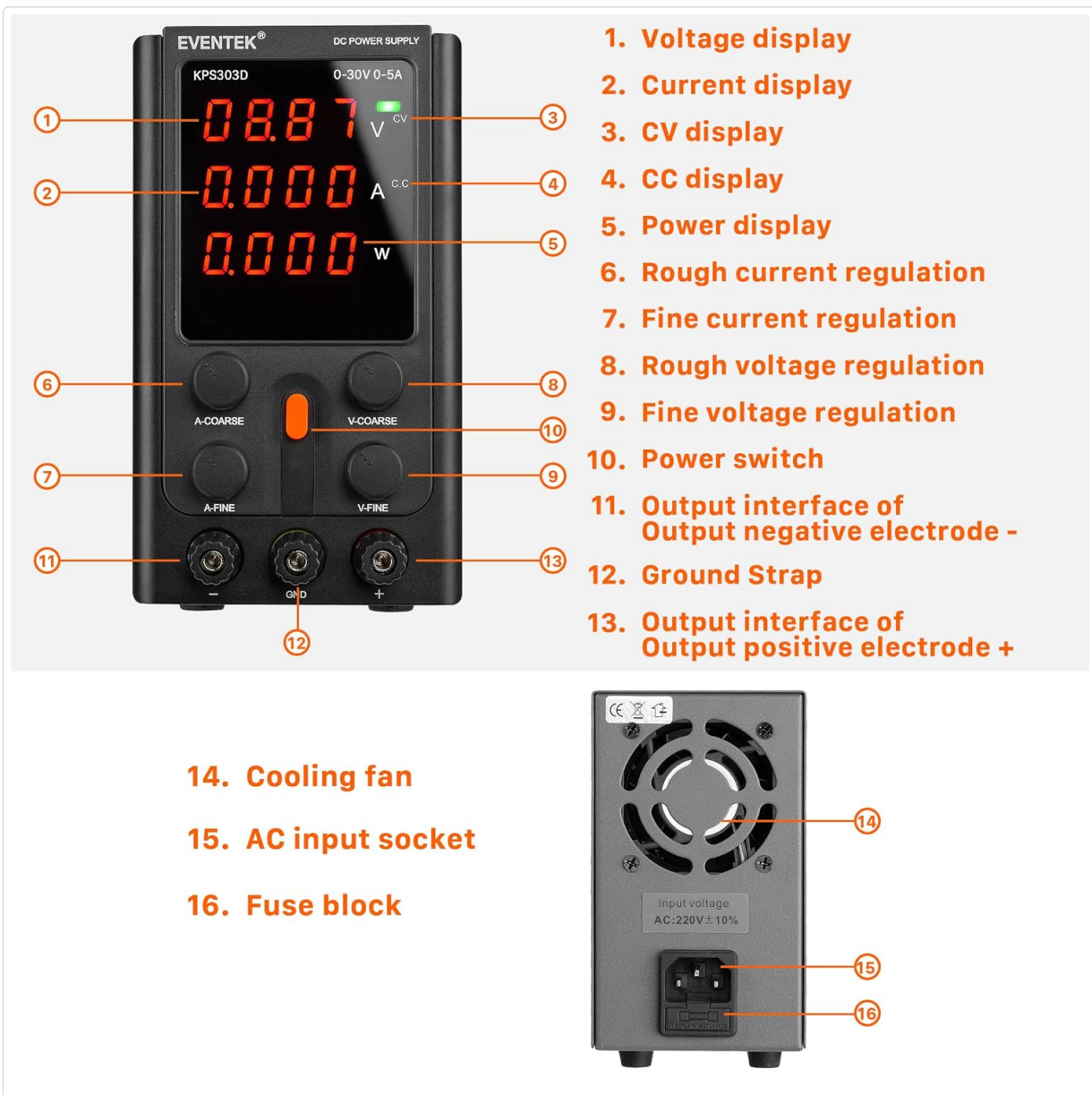
Figure 3: Detailed diagram of the power supply's front and rear panel components.
