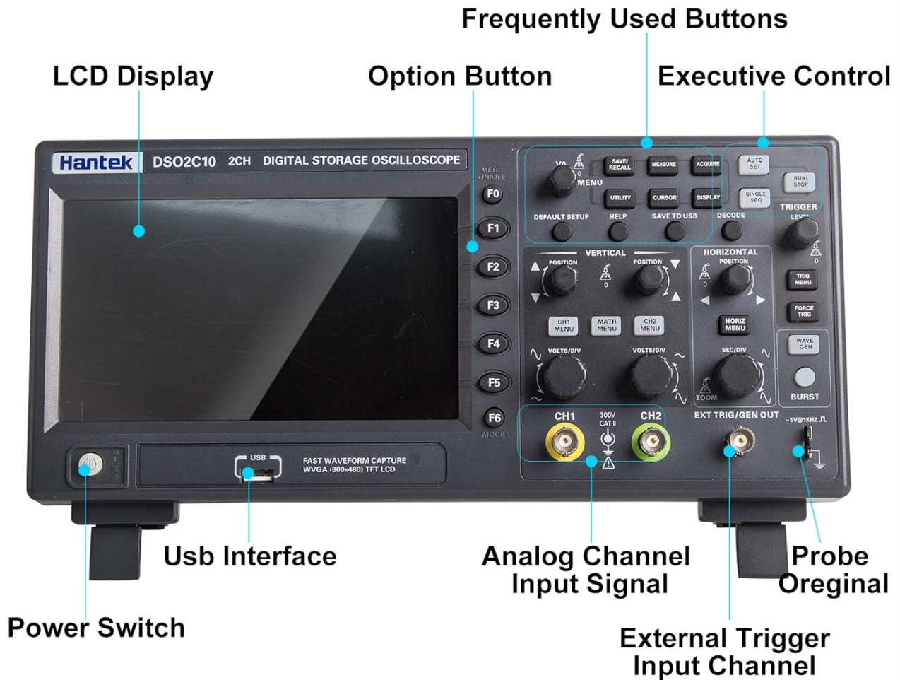
Figure 4.1: Detailed view of the Hantek DSO2C10 front panel, highlighting the LCD Display, Option Buttons (F1-F6), Executive Controls (e.g., MENU, UTILITY, CURSOR, DISPLAY, SAVE TO USB, DECODE, TRIGGER LEVEL), Vertical and Horizontal controls, Analog Channel Input Signals (CH1, CH2), External Trigger Input Channel, USB Interface, and Power Switch.
