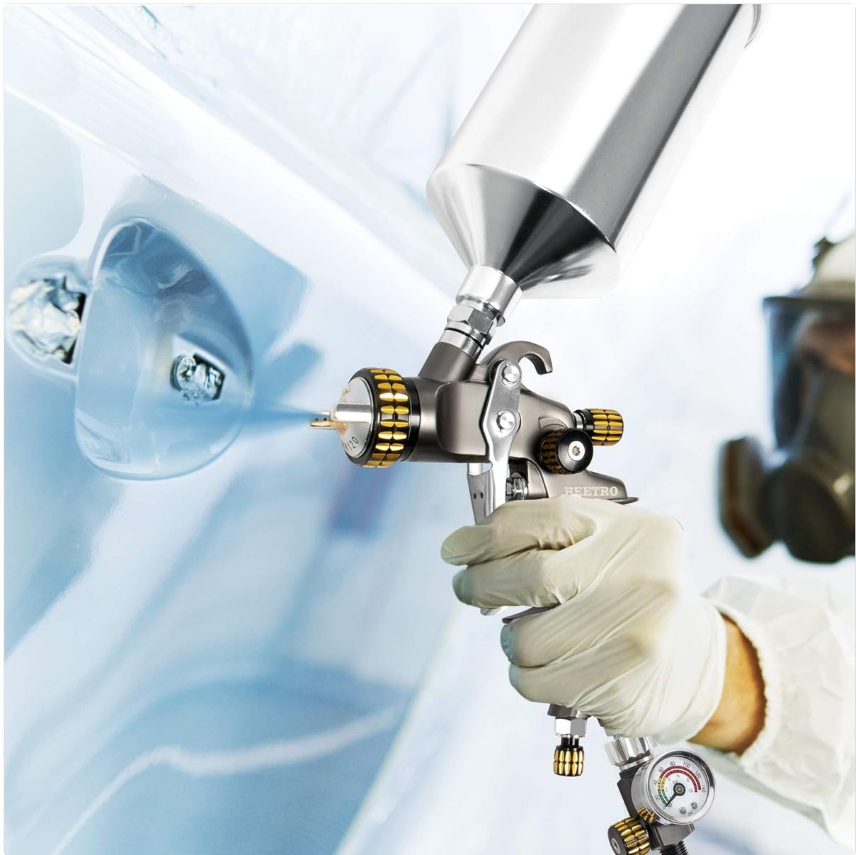
Figure 6: The spray gun in action, demonstrating its use for applying coatings to a surface.
