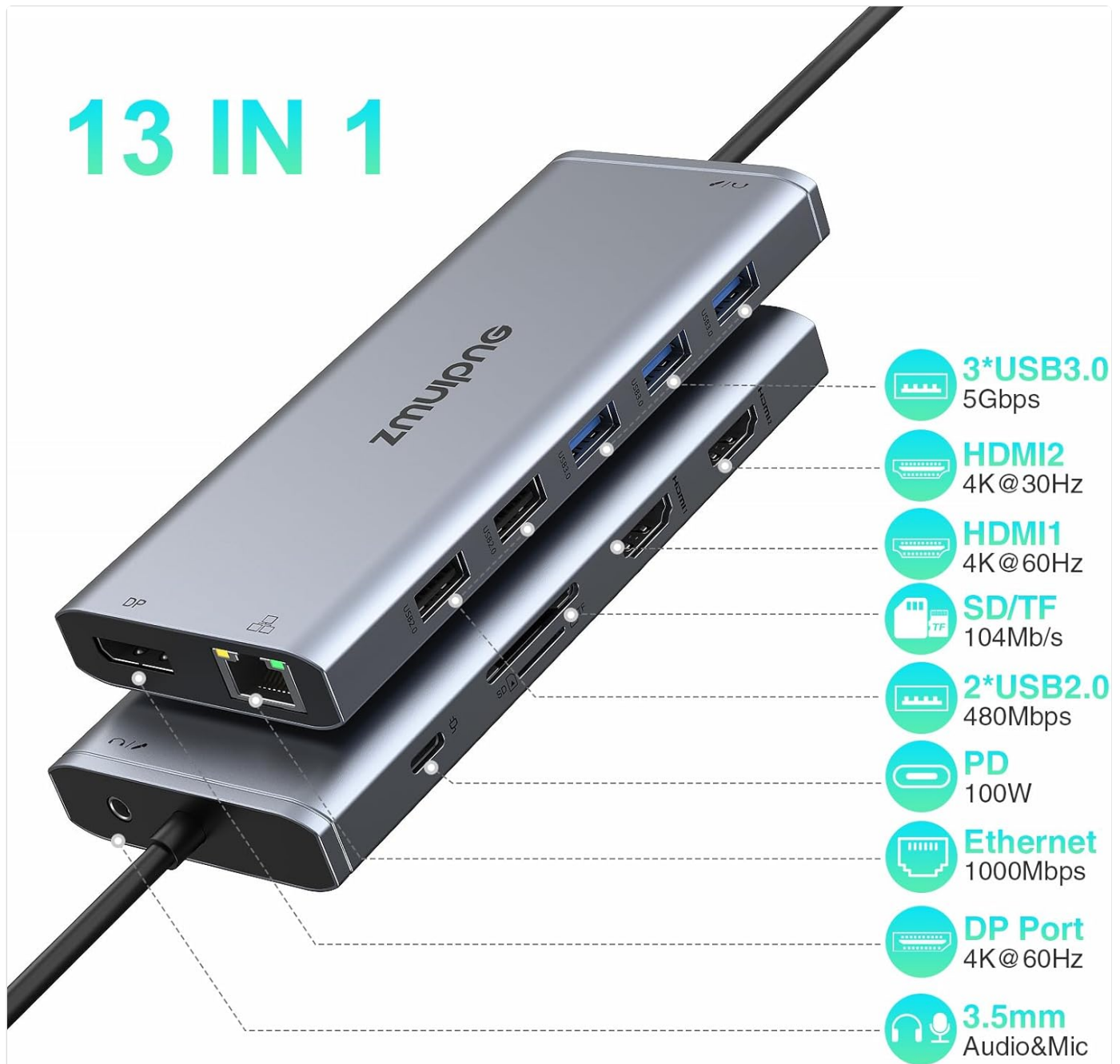
Image: A detailed diagram illustrating the various ports of the ZMUIPNG docking station, including 3x USB 3.0, 2x HDMI, SD/TF card slots, 2x USB 2.0, PD 100W, Ethernet, DP Port, and 3.5mm Audio/Mic.
