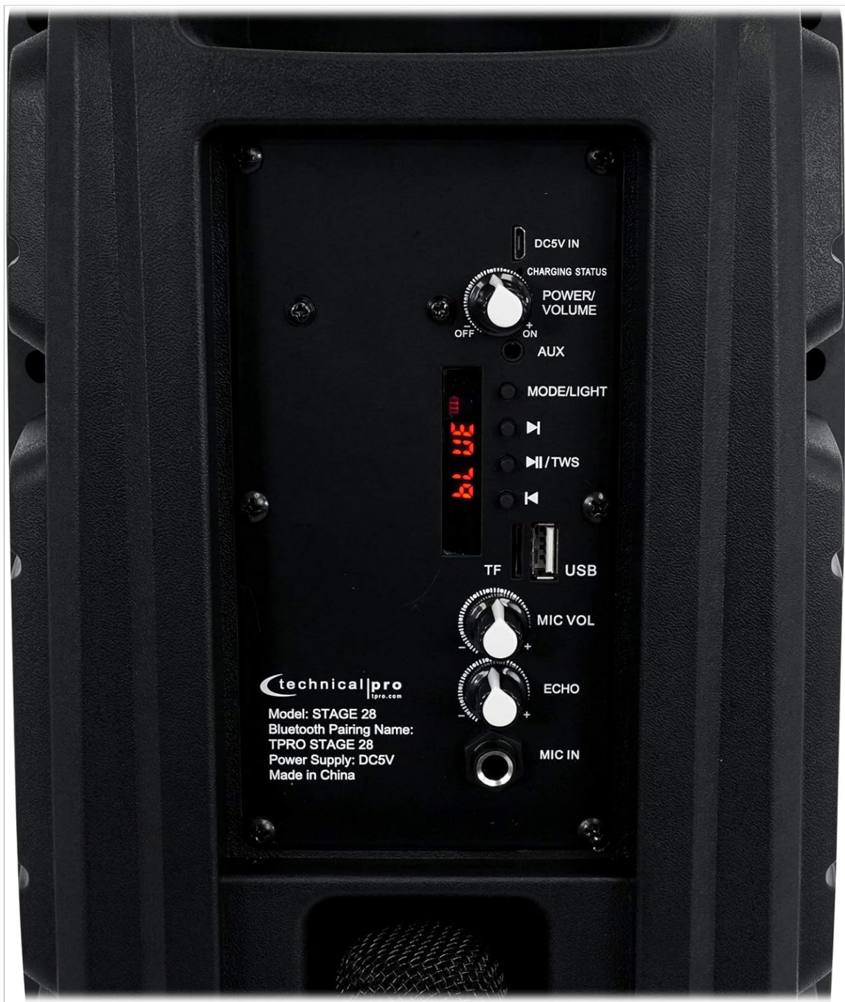
Image: Rear control panel detail, highlighting the DC5V IN port.
