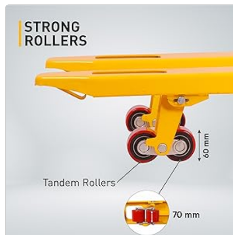
Figure 3.2: Detail of the tandem rollers (bogie wheels) located under the forks, designed for smooth movement over uneven surfaces and reduced wear.
