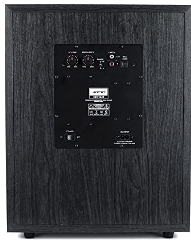
Figure 3: Jamo C912 Subwoofer Rear Panel. This image details the rear panel of the subwoofer, showing the various input connections and control knobs for volume, frequency (crossover), and phase adjustment, along with the power switch and AC input.
