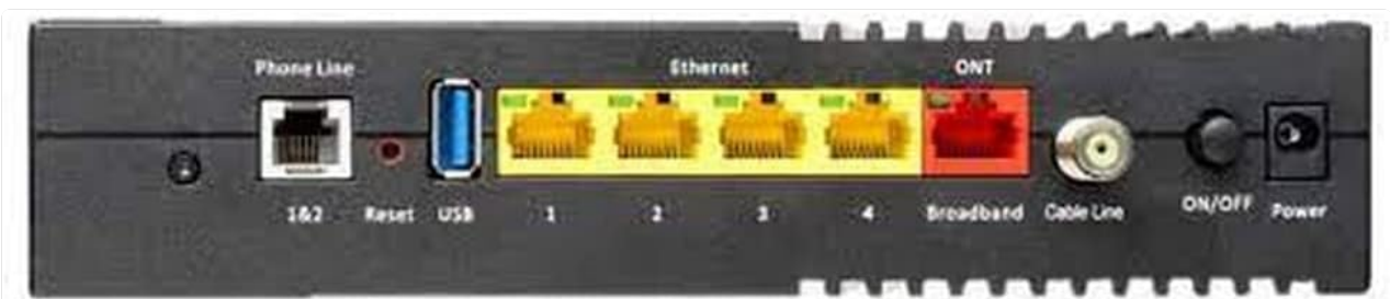
Figure 1: Rear view of the Arris NVG468MQ showing various connection ports including Phone Line, Ethernet, ONT, Cable Line, and Power.
