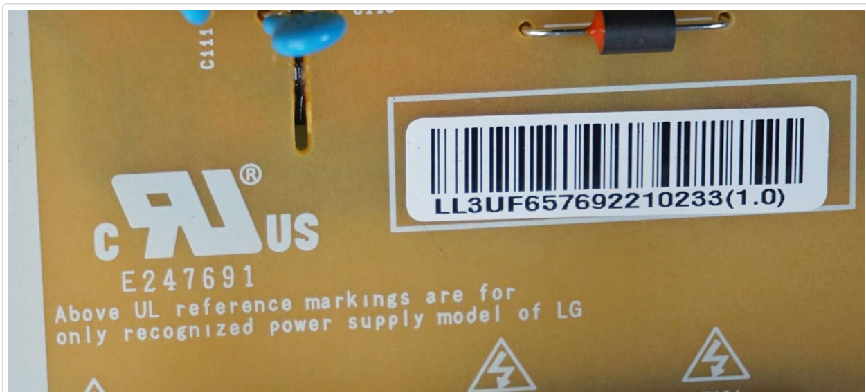
Figure 3.7: View of the UL reference markings and another instance of the barcode for model number LL3UF657692210233 , indicating compliance and aiding in part verification.
