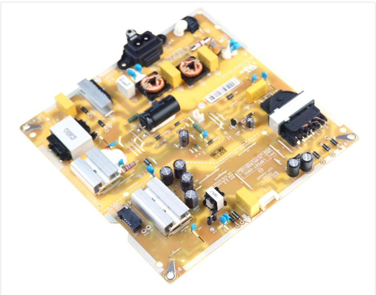
Figure 3.1: Top view of the R22 Power Supply Board, showing various components and connectors. This perspective helps in identifying the overall layout and component placement.
