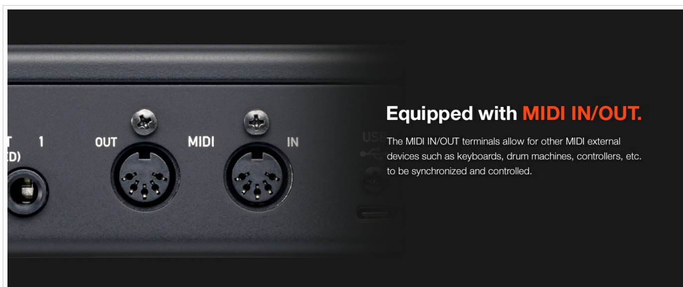
Figure 3.6.1: MIDI IN/OUT ports for connecting external MIDI devices.
