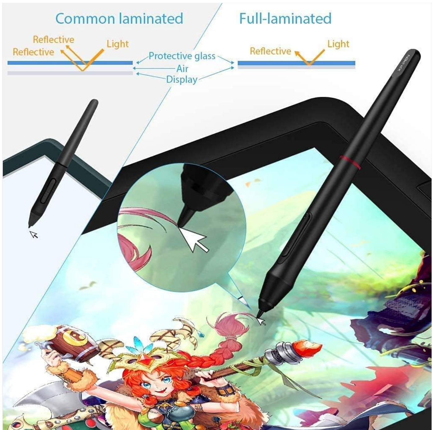
Figure 3.1: Illustration of the difference between common laminated and full-laminated display technologies, highlighting reduced reflection and improved visual clarity with full lamination.
