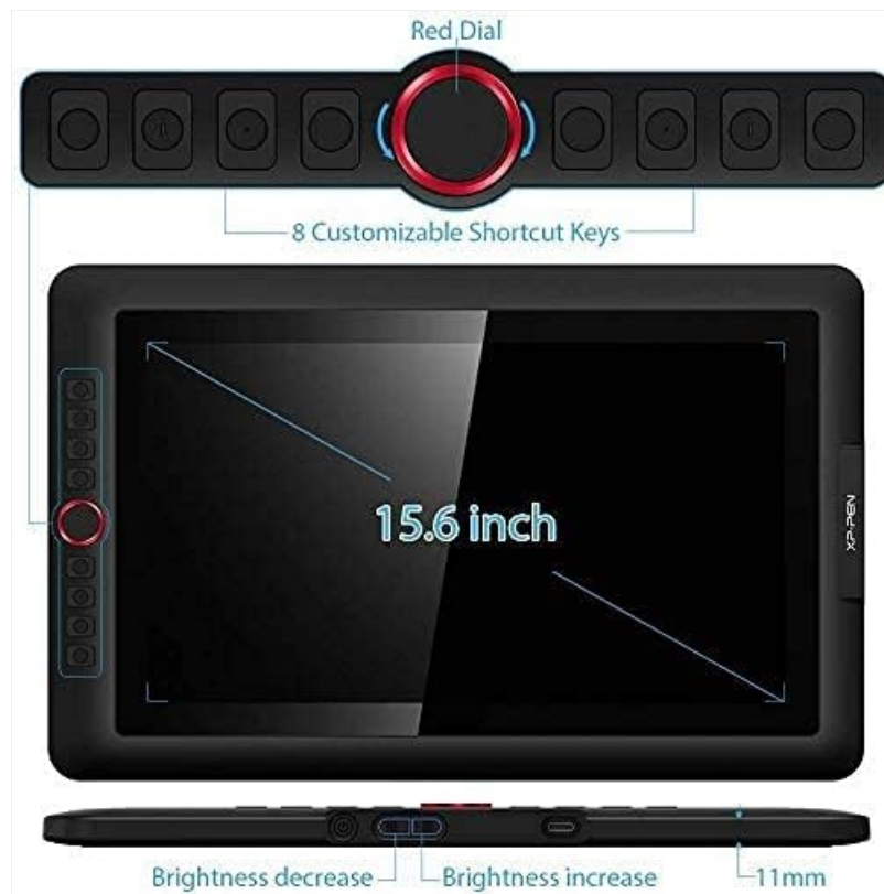
Figure 3.4: Overview of the Artist15.6 Pro, highlighting the Red Dial, 8 customizable shortcut keys, and brightness adjustment buttons.
