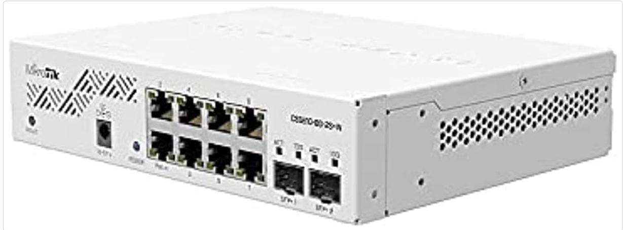
Figure 4.1: Angled front view of the MikroTik CSS610-8G-2S+IN Cloud Smart Switch, showing the eight Gigabit Ethernet ports, two SFP+ ports, power input, and reset button.
