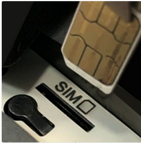
Image: A close-up view of the SIM card slot, indicating where the Nano-SIM card is inserted.
