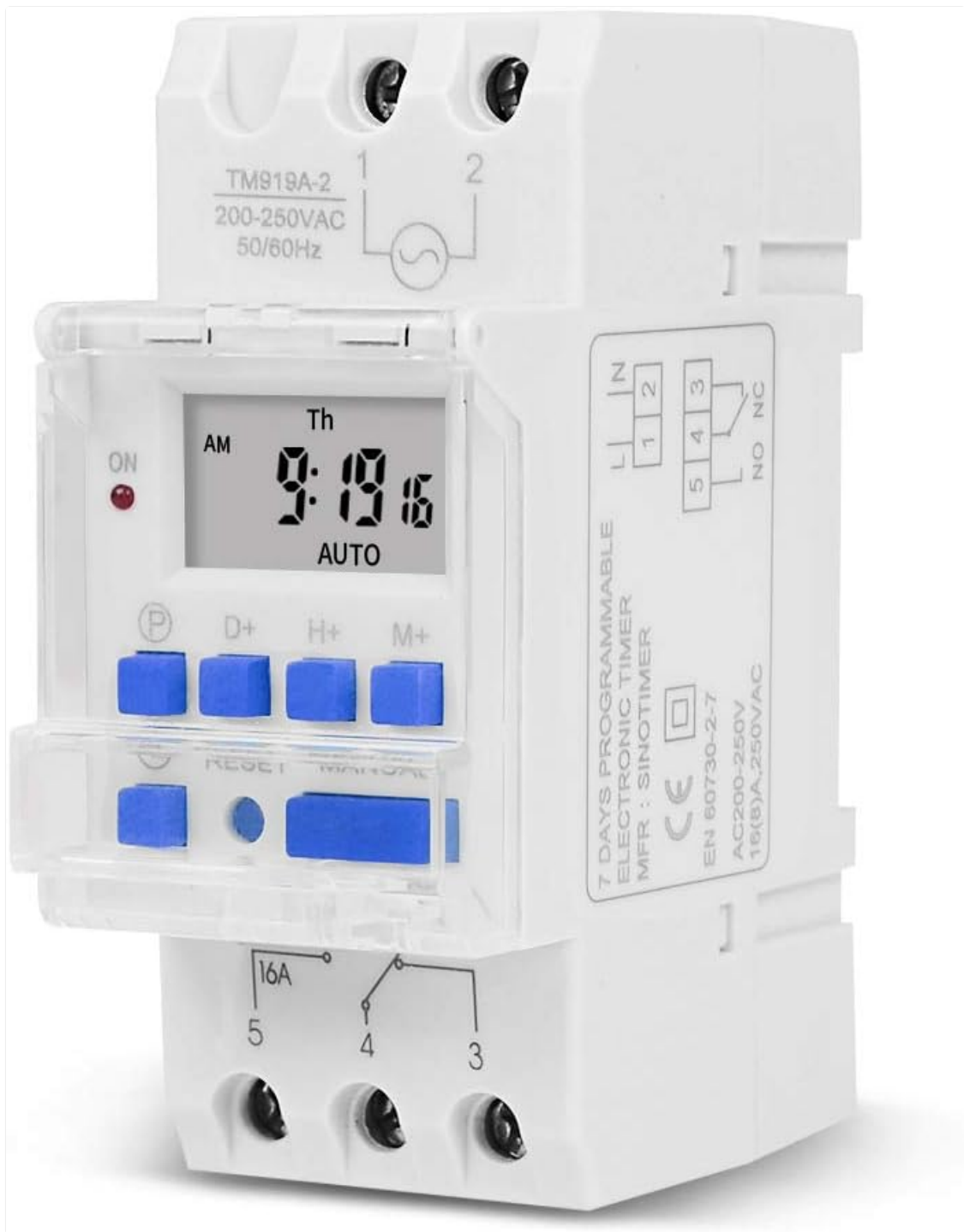
Figure 5.1: Side view of the timer switch displaying the wiring diagram. Terminals 1 and 2 are for power input (L and N). Terminals 3, 4, and 5 are for the relay output (Common, Normally Open, Normally Closed).
