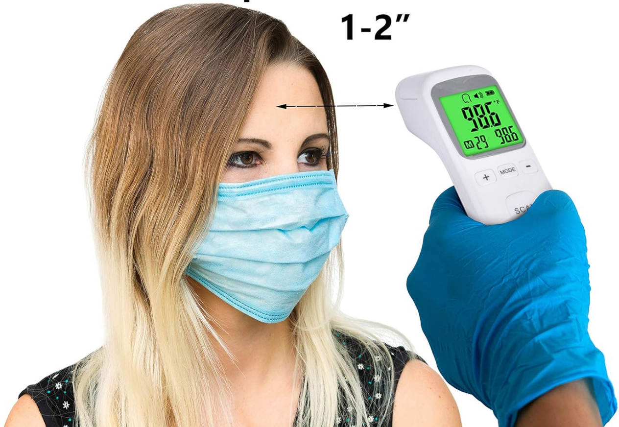
Figure 6.1: The three-color LCD display indicating temperature ranges for normal, slight fever, and high fever.
