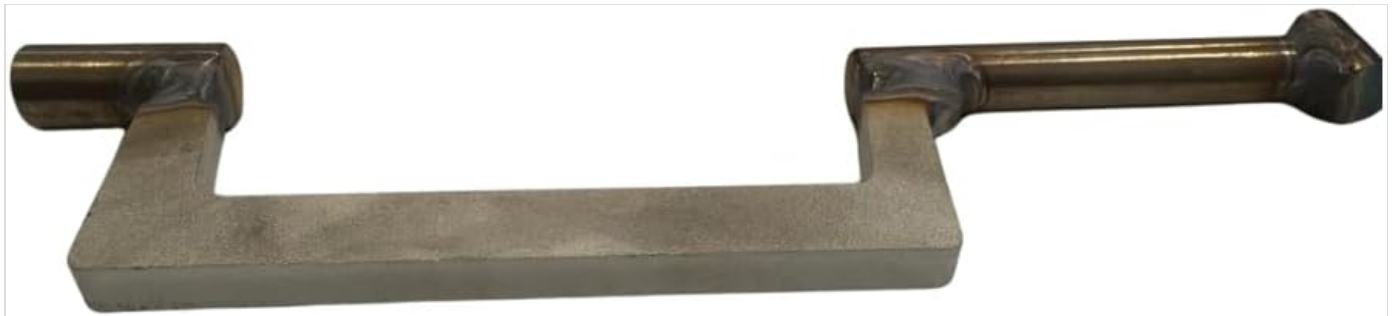
Image 3: Top-down view of the Thermorossi scraper tool. This image provides a clear perspective of the tool's overall length and the distinct L-shaped scraping blade, with cylindrical handles at each end.
