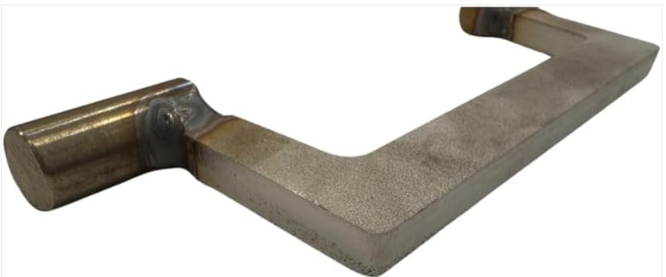
Image 2: Angled close-up view of one end of the Thermorossi scraper tool. This perspective highlights the cylindrical handle section and the weld connecting it to the main scraping blade.
