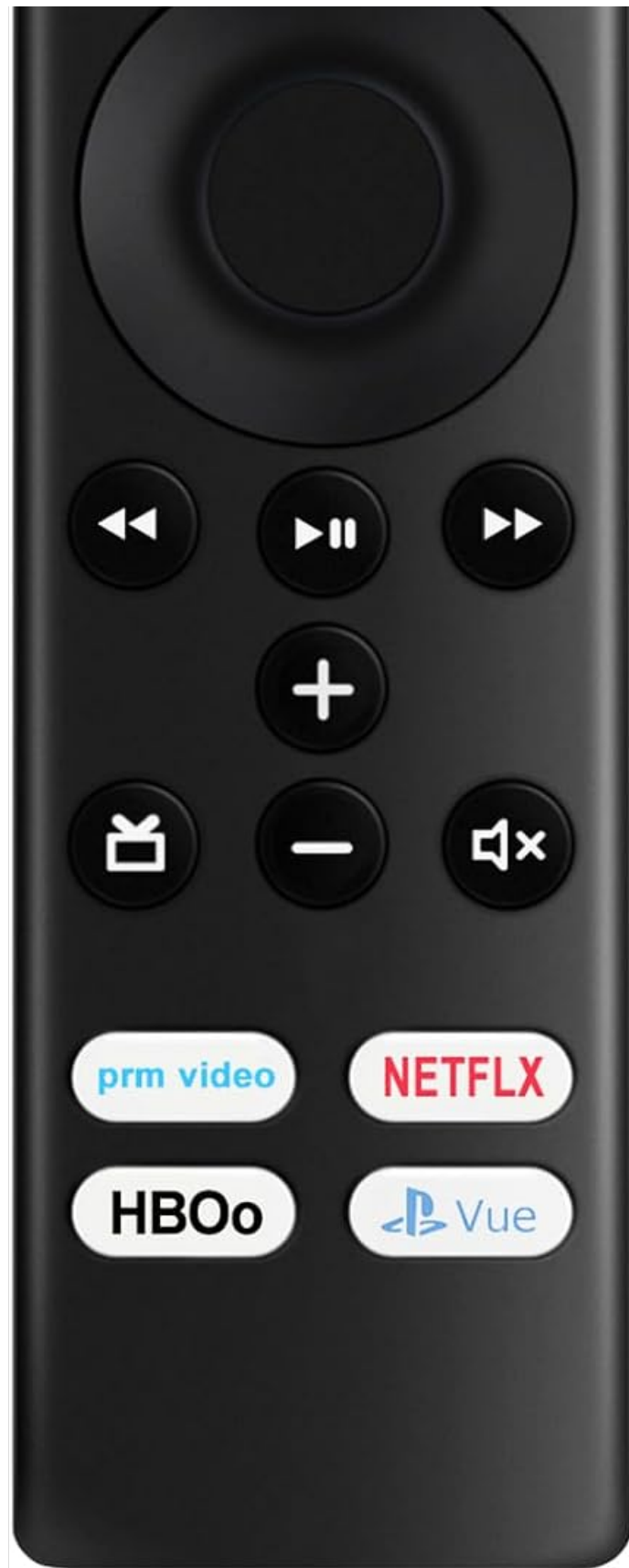
Figure 1: Front view of the ZdalaMit CT-RC1US-19 Voice Remote Control, showing all buttons including power, voice, navigation, playback, volume, and dedicated app buttons.
