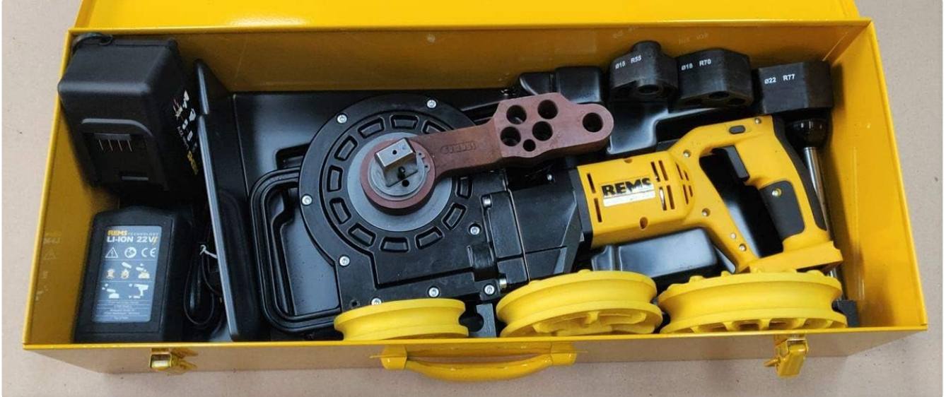
Image 3: Close-up view of the bending segments (black, marked with diameters like Ø15 R55, Ø18 R70, Ø22 R77) and the yellow sliding pieces, along with the main bending mechanism of the REMS Curvo 22 V.
