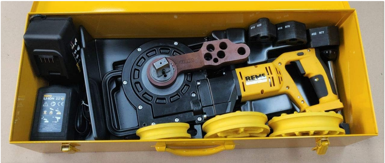
Image 4: The main yellow and black REMS Curvo 22 V pipe bending tool, showing its ergonomic design and the central bending mechanism.
