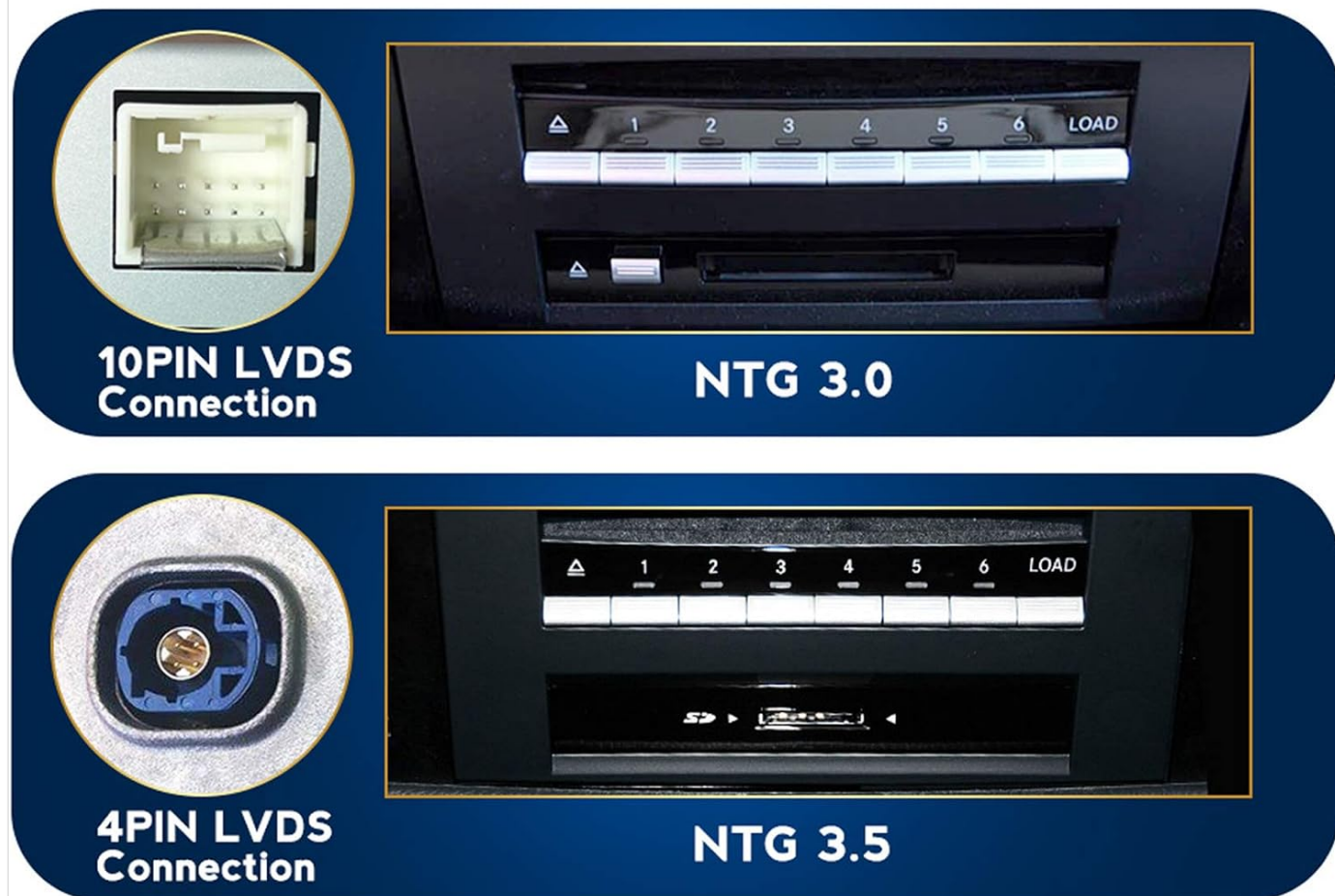
Figure 2: Identifying NTG 3.0 (10PIN LVDS) and NTG 3.5 (4PIN LVDS) connections.
