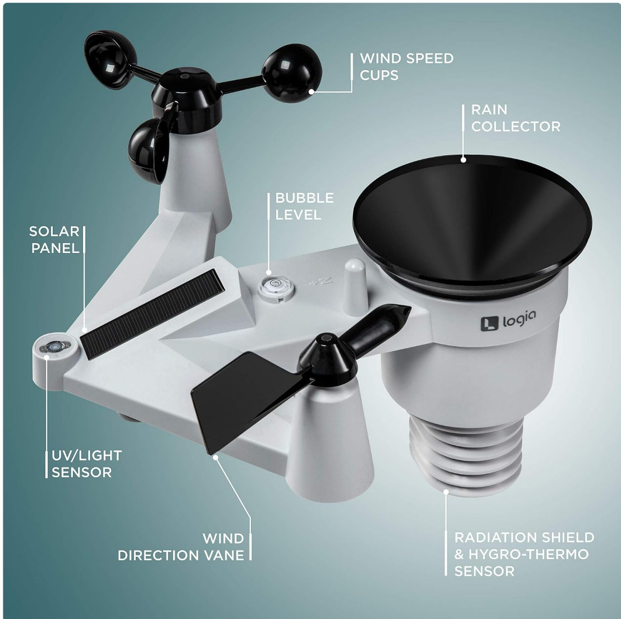
Figure 2: Outdoor 7-in-1 Sensor Array components.
