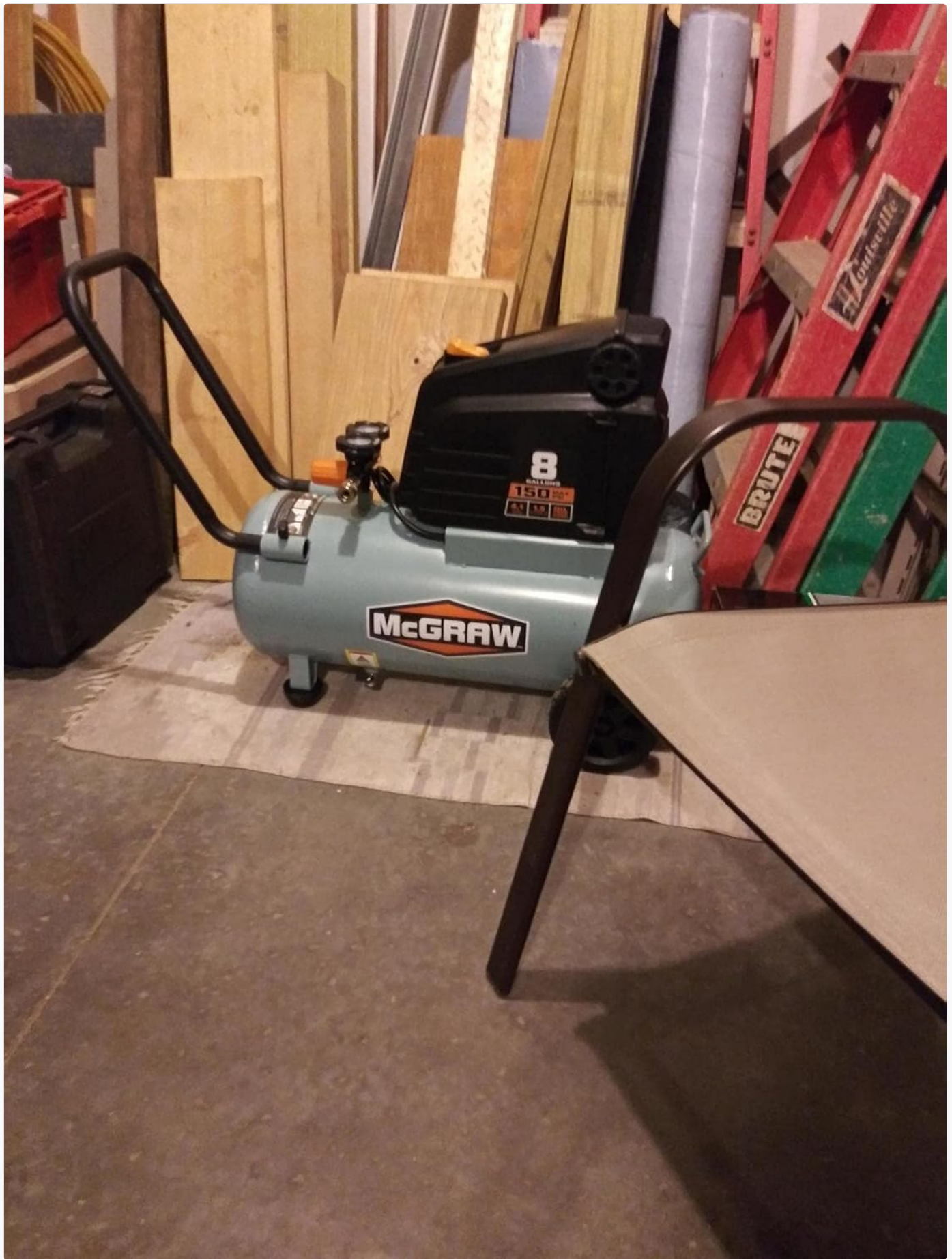
An image showing the HFT 8 Gallon 1.5 HP 150 PSI Oil-Free Portable Air Compressor. The compressor features a light blue tank, a black motor housing on top, a black handle, and wheels for portability. Gauges and a quick connect coupler are visible on the front.
