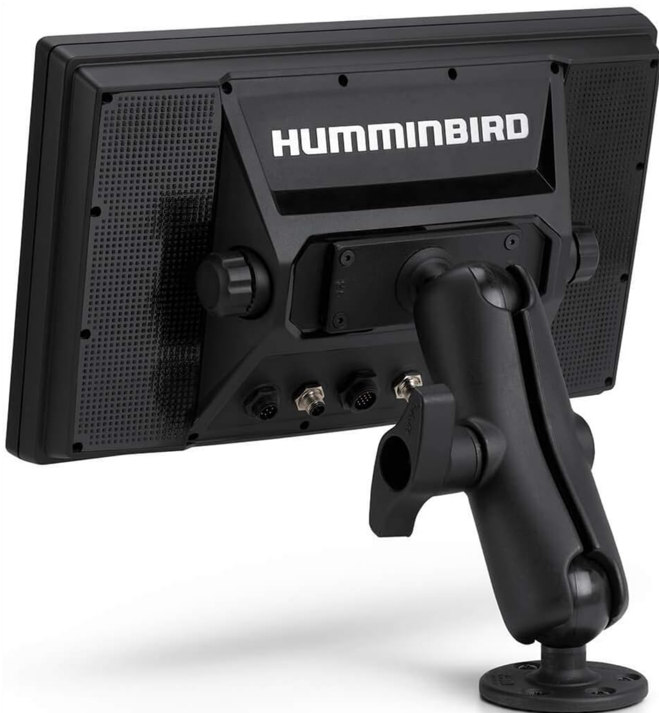
Image: Side view of the SOLIX 15 unit showing the mounting bracket.
