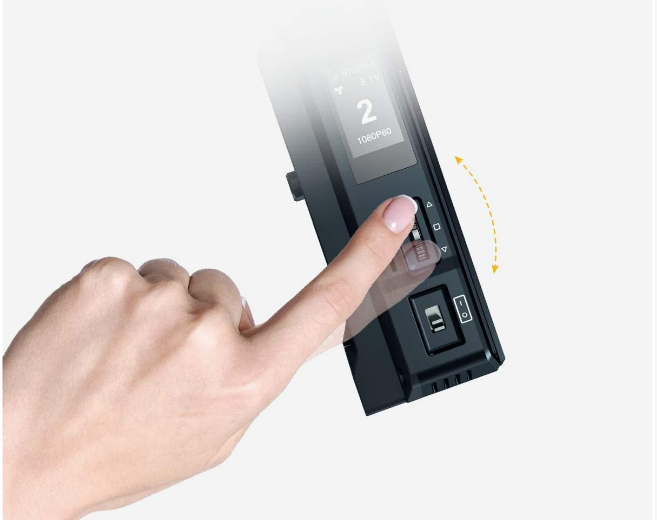
Figure 5.1: A hand interacting with the thumbwheel switch menu on the Mars 300 PRO. The thumbwheel is used to navigate and select options displayed on the side OLED screen, enhancing user experience.
