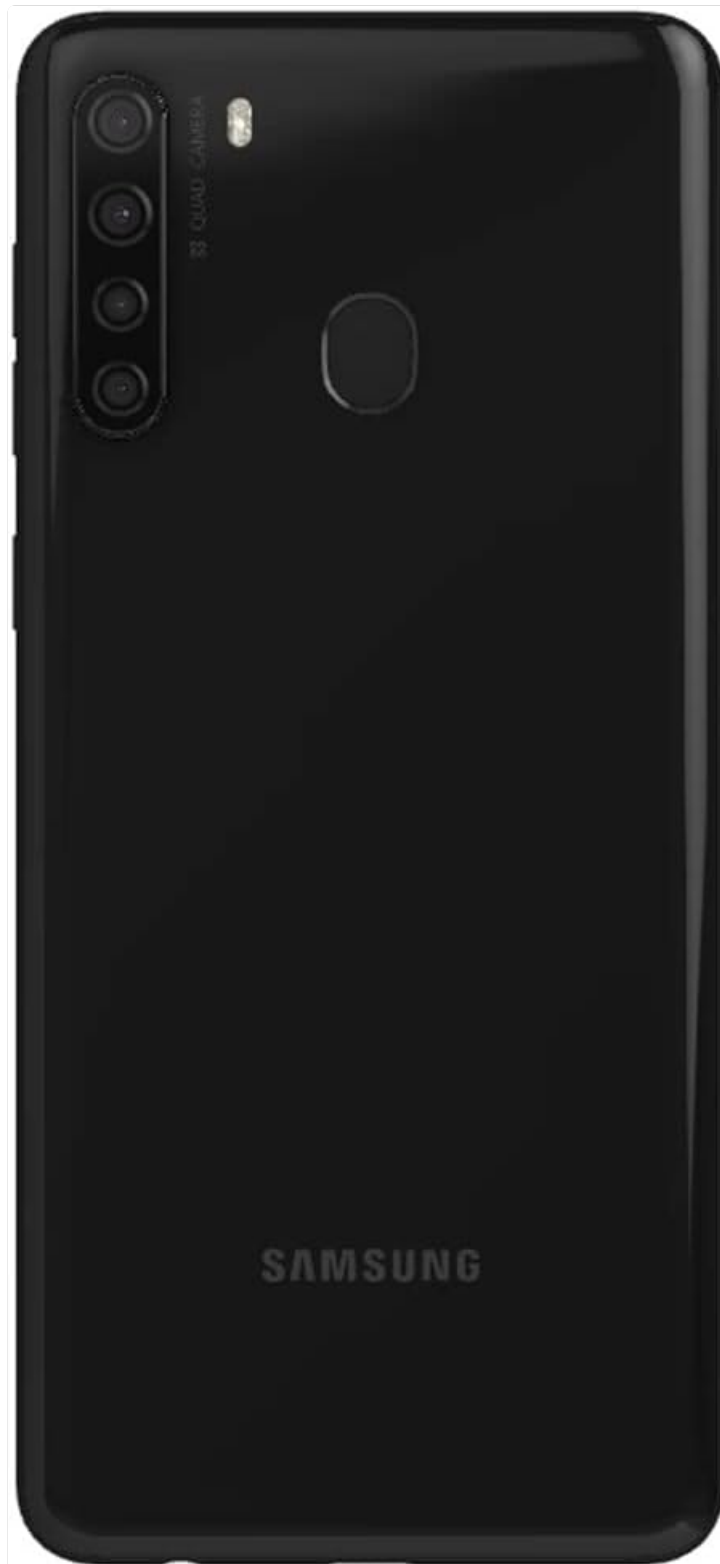
Figure 4: Back view of the Samsung Galaxy A21, highlighting the quad-camera system and fingerprint sensor.
