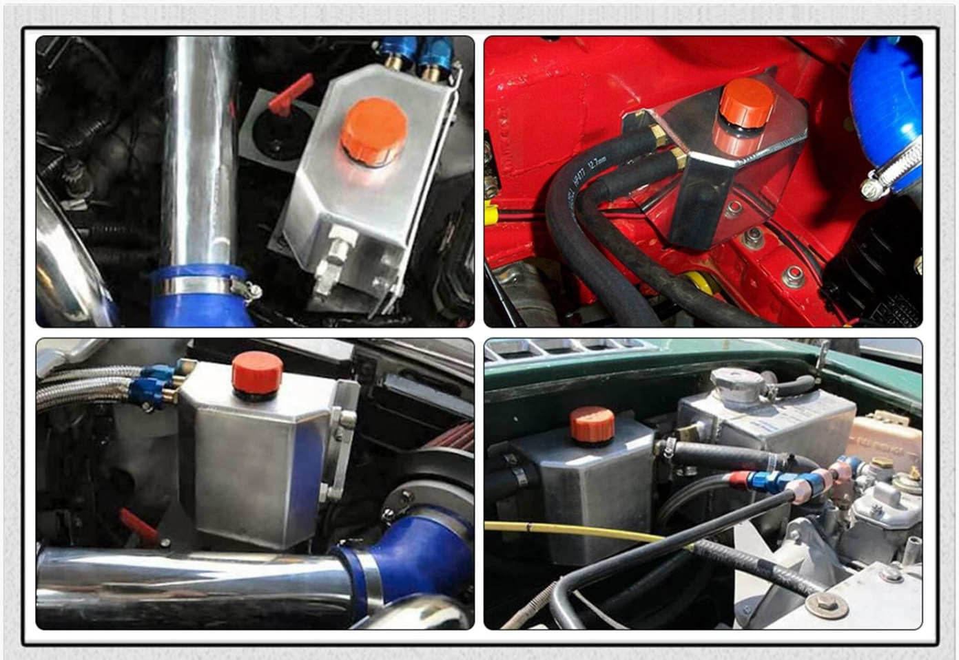
Figure 4.1: Examples of oil catch can installations. This collage shows the catch can installed in different vehicle engine compartments, demonstrating various mounting positions and hose routing possibilities. These are illustrative examples and actual installation may vary based on vehicle type.
