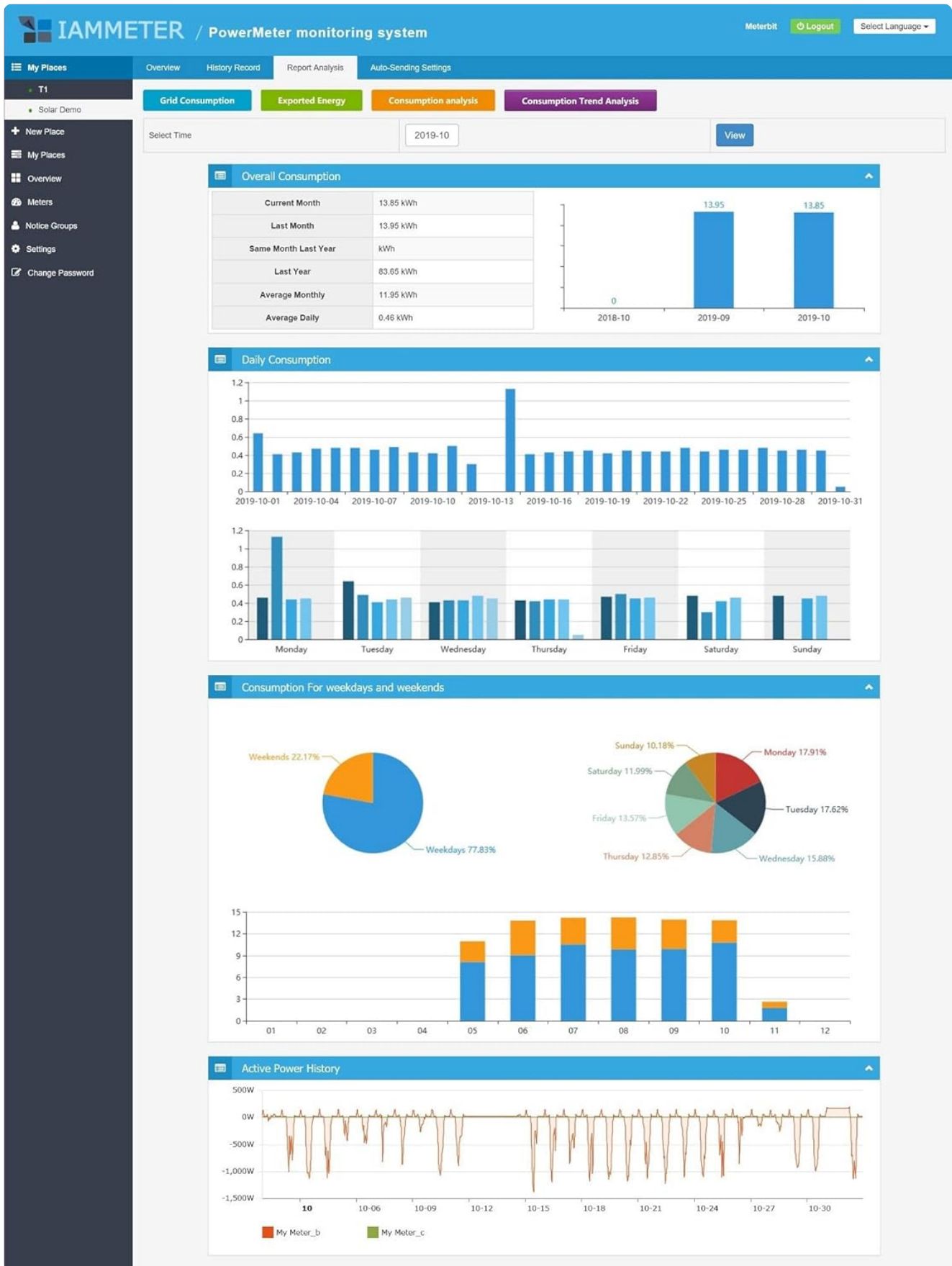
Image: Screenshot of the IAMMETER web monitoring interface for a residential system, showing power consumption trends, daily/monthly/yearly energy usage, and location-based weather information.
