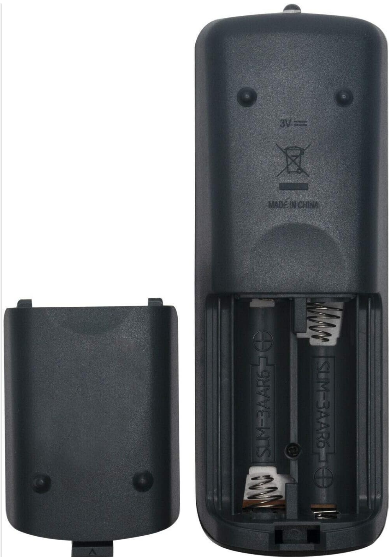
Figure 2.1: Battery compartment of the RM-AMU053 remote control.
