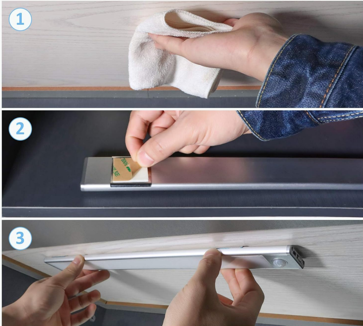
Image 4.1.1: Step-by-step visual guide for installing the light: 1. Cleaning the surface, 2. Attaching the adhesive metal sheet, 3. Magnetically mounting the light bar.
