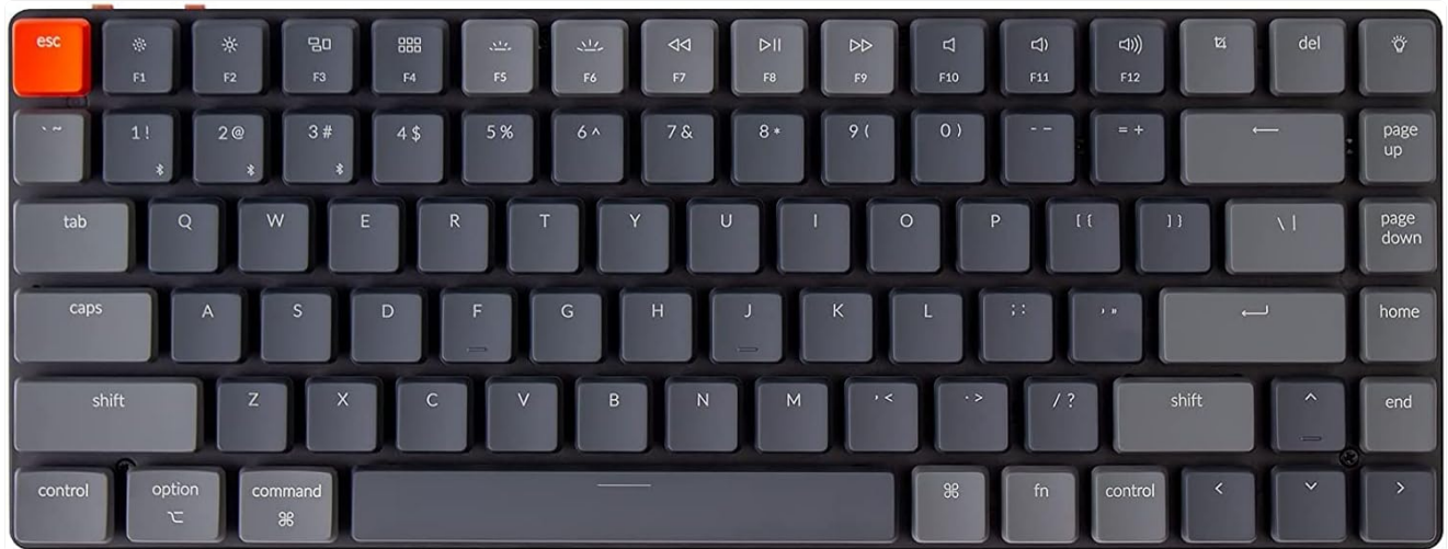
Figure 1: Top-down view of the Keychron K3 keyboard, highlighting its compact 75% layout.
