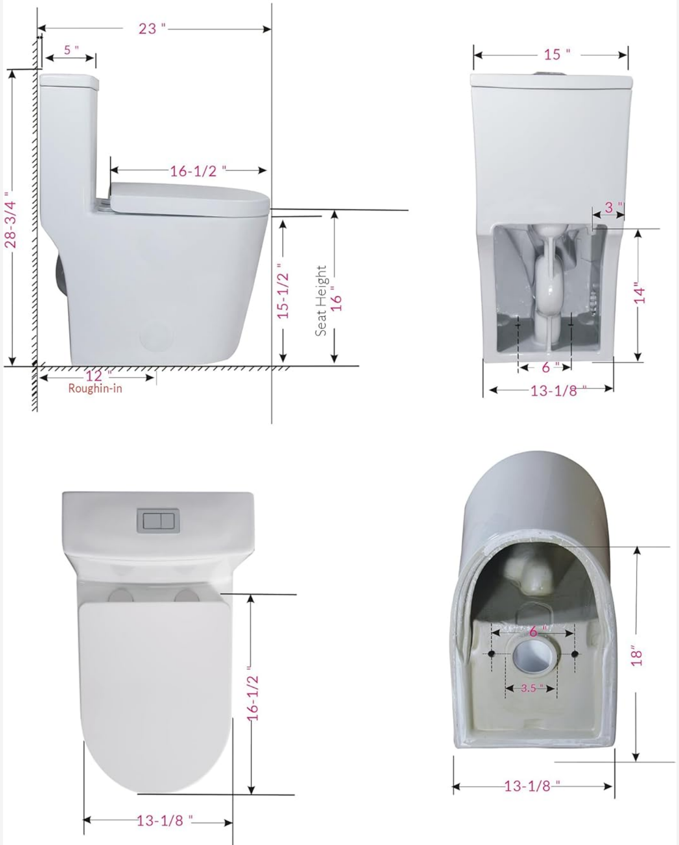
Figure 3.1: Product Dimensions. This diagram provides detailed measurements including depth (23"), width (15"), height (28.75"), seat height (16"), and 12" rough-in.
