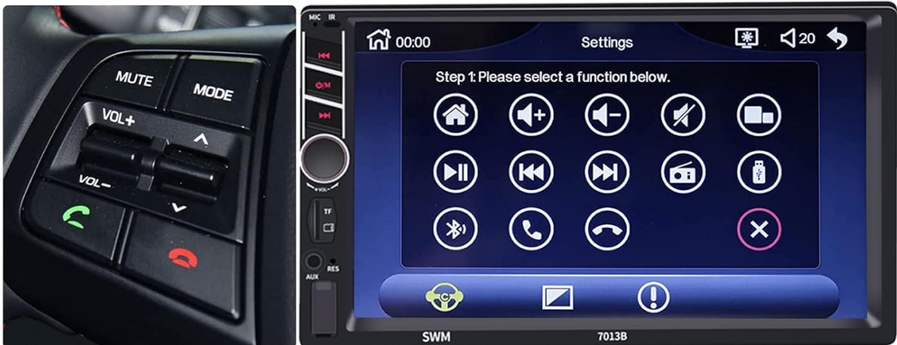
Figure 4.6: The steering wheel control setup interface, allowing users to map various functions to their vehicle's steering wheel buttons.
