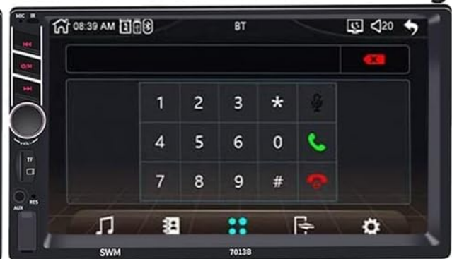
Figure 4.2: The Bluetooth connection screen, showing options for Bluetooth music playback and hands-free calling with a dial pad.
