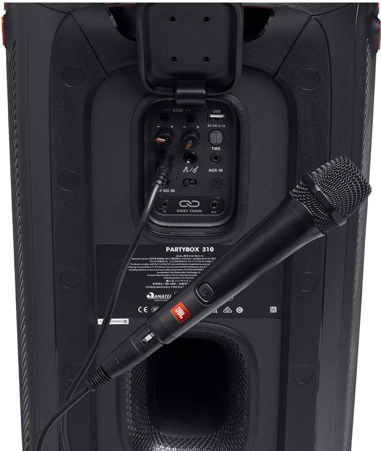
The JBL PartyBox Mic 100 connected to the 6.35mm microphone input on the rear panel of a JBL PartyBox 310 speaker, demonstrating a typical setup.
