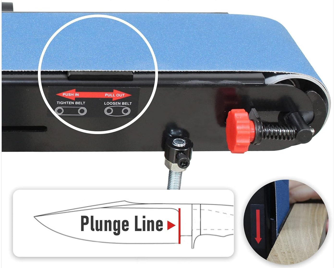
Figure 7: Plunge line sharpening accessory for knife grinding.
