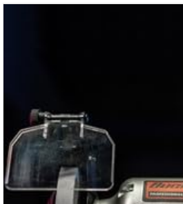
Figure 13: Belt tension adjustment knob.
