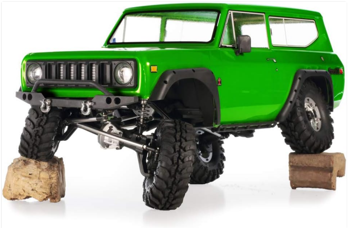
Figure 5: The truck's suspension articulation shown over uneven terrain.
