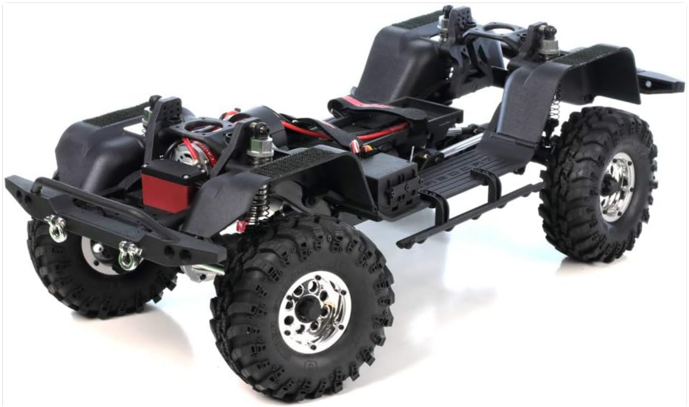
Figure 2: The robust chassis of the Gen8 V2, highlighting its C-channel frame rails and suspension components.
