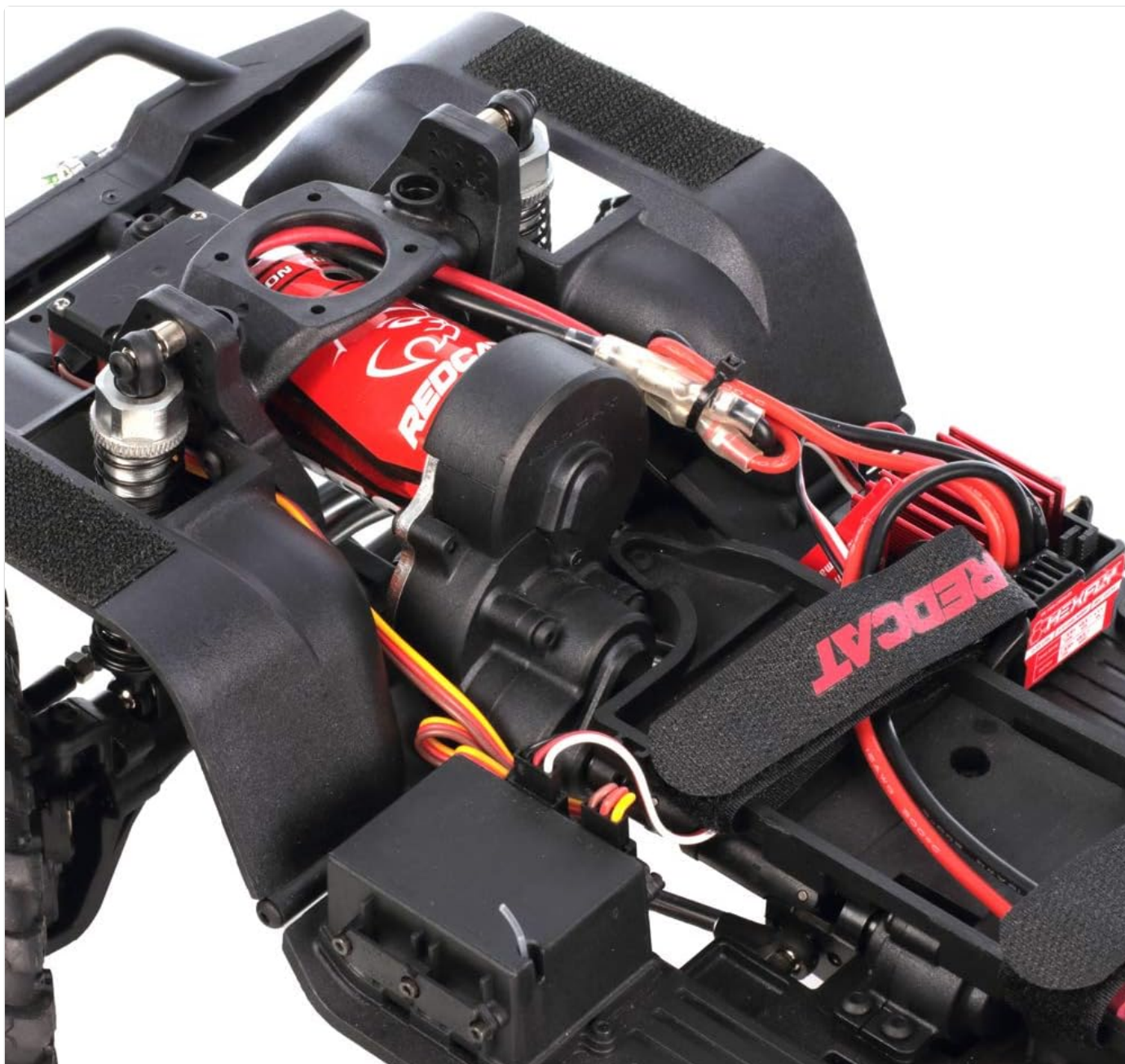
Figure 3: Close-up view of the front-mounted motor and wiring, showing the battery connection area.
