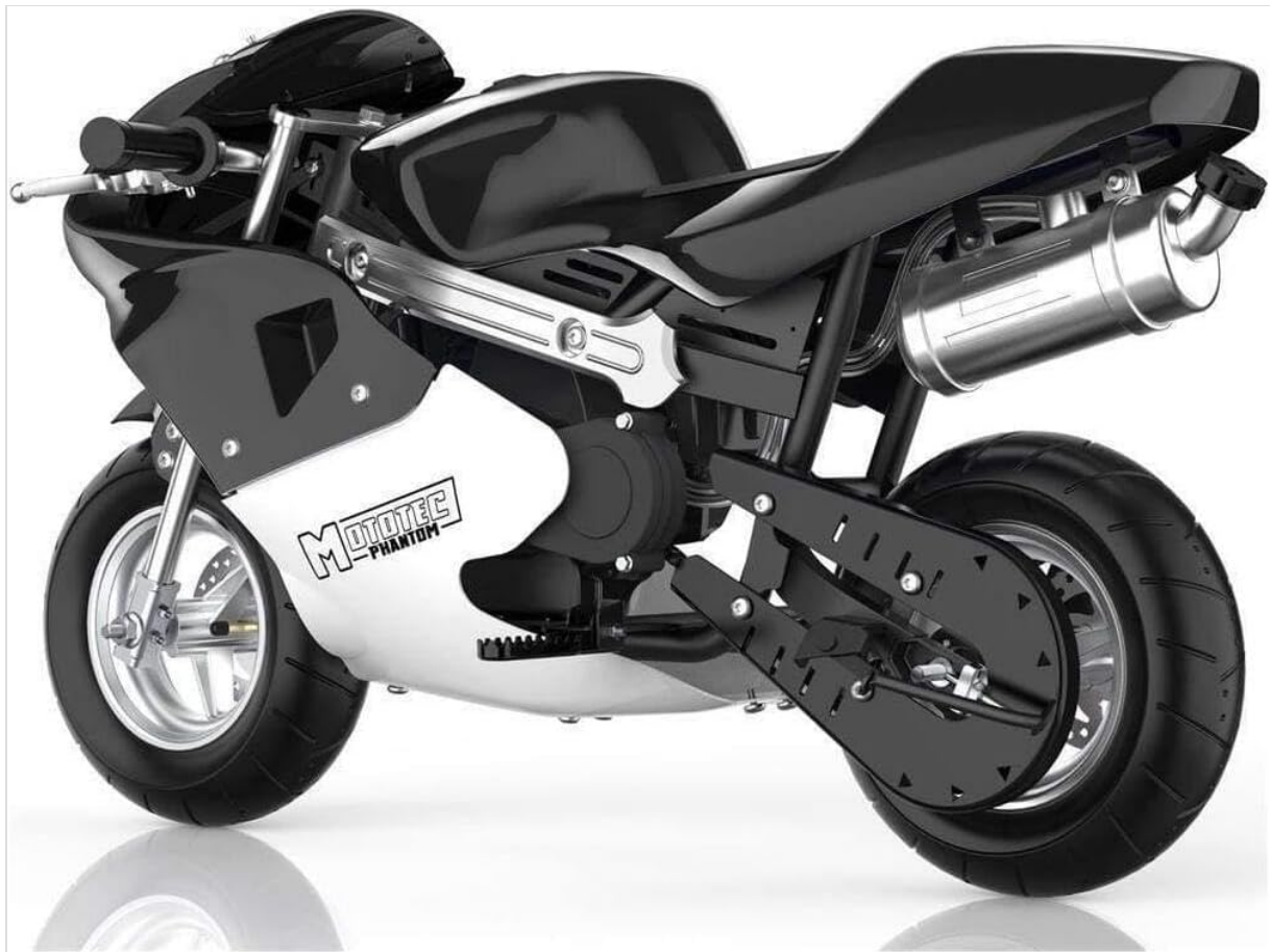
Image: Rear view of the MotoTec Phantom pocket bike, showing the rear wheel, chain, and disc brake.
