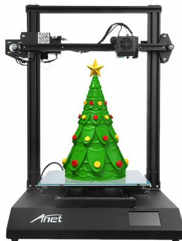
Image 2.3: The Anet ET5 Pro integrates a 350W Meanwell power supply, concealed within the machine for convenience and safety.
