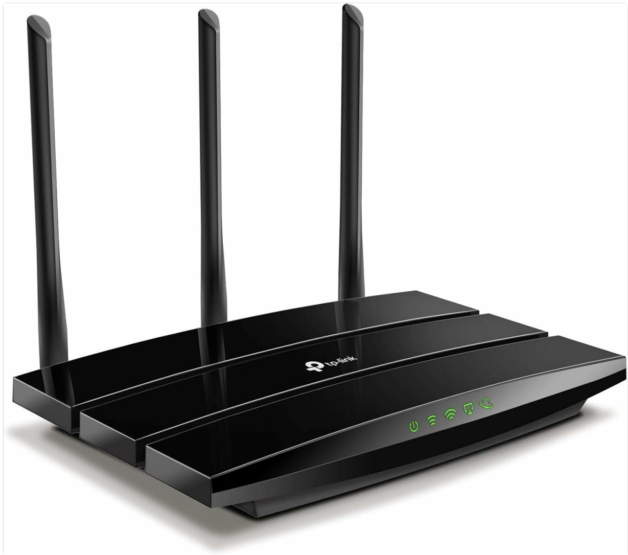
Figure 3.1: Front View of TP-Link Archer A8 Router. This image displays the top-down view of the TP-Link Archer A8 router, featuring its sleek black design and three external antennas. The front panel includes LED indicators for power, internet connectivity, Wi-Fi status, and Ethernet port activity.
