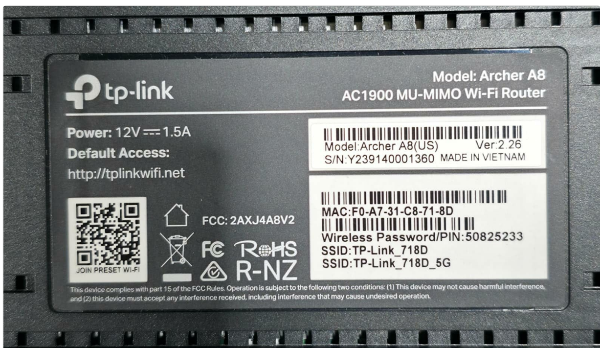
Figure 3.3: Router Bottom Label. This label provides essential information including the model (Archer A8, AC1900 MU-MIMO Wi-Fi Router), power specifications (12V===1.5A), default access URL ( http://tplinkwifi.net ), MAC address
