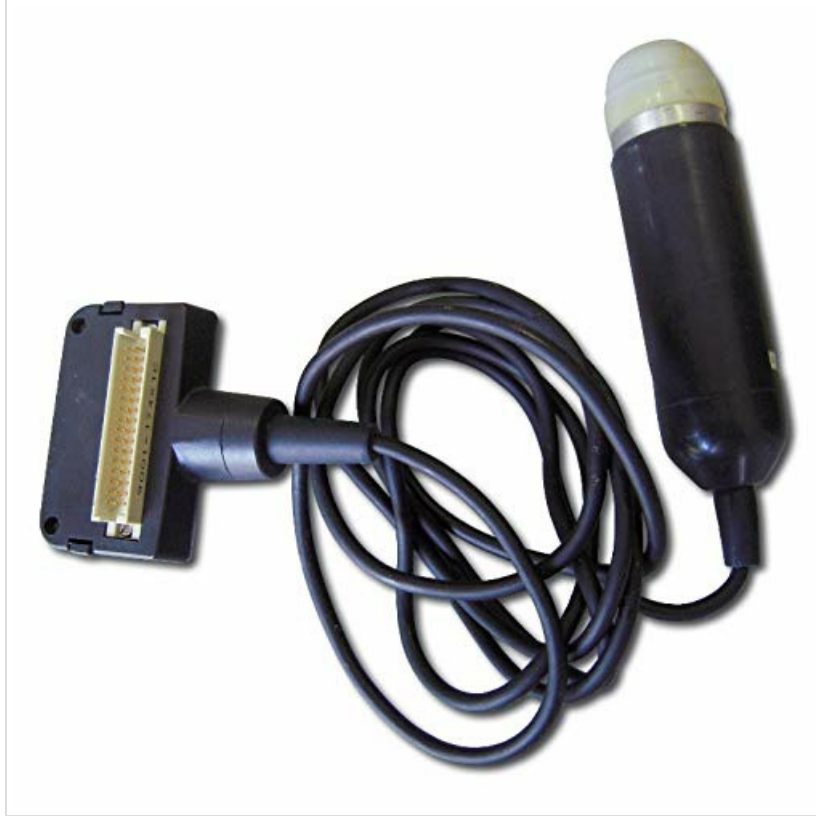
Image 2.1: The 3.5 MHz mechanical sector probe with its connecting cable.
