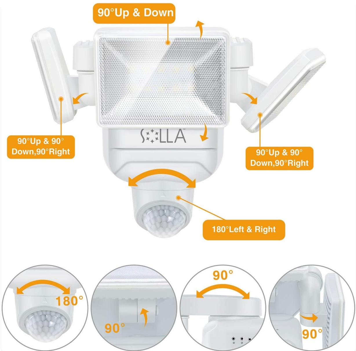
This diagram illustrates the adjustable features of the SOLLA solar light. It shows that the three light heads can be adjusted 90 degrees up and down, and 90 degrees left and right. The motion sensor itself can be rotated 180 degrees left and right, allowing for precise targeting of both light and detection areas.
