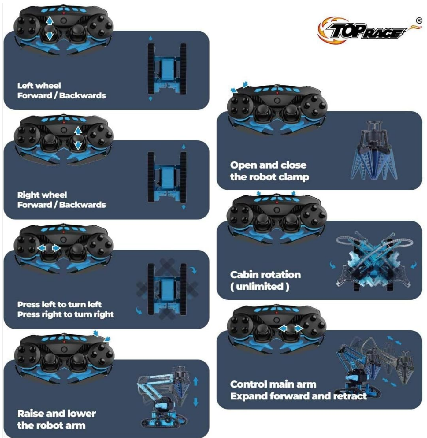
Figure 5.1: This diagram illustrates the various control inputs on the remote control and their corresponding actions on the robotic arm. It shows controls for track movement, arm articulation, cabin rotation, and gripper operation.
