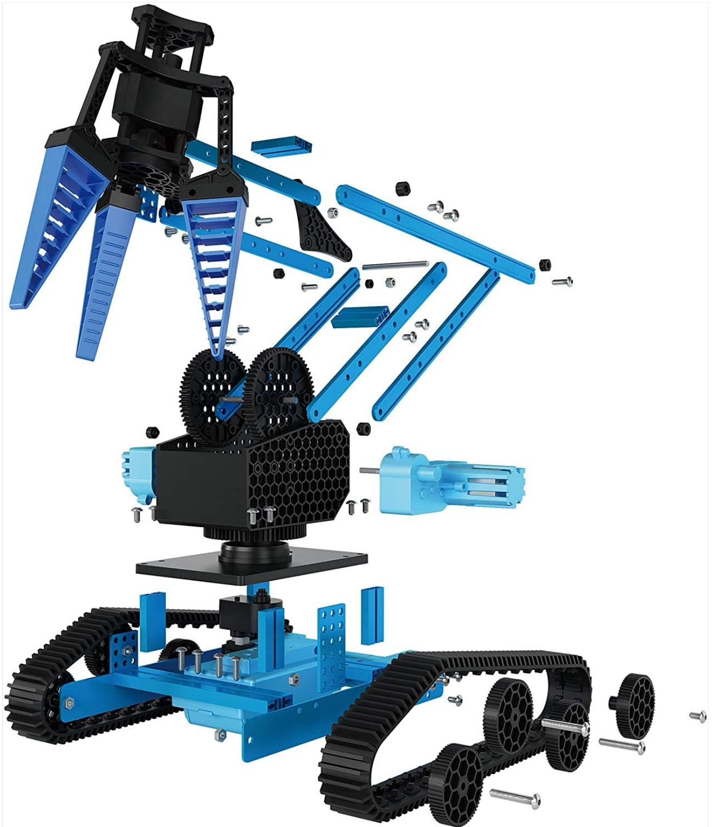
Figure 4.1: An exploded diagram illustrating the various parts of the robotic arm and their relative positions before assembly. This view helps in understanding the construction process.
