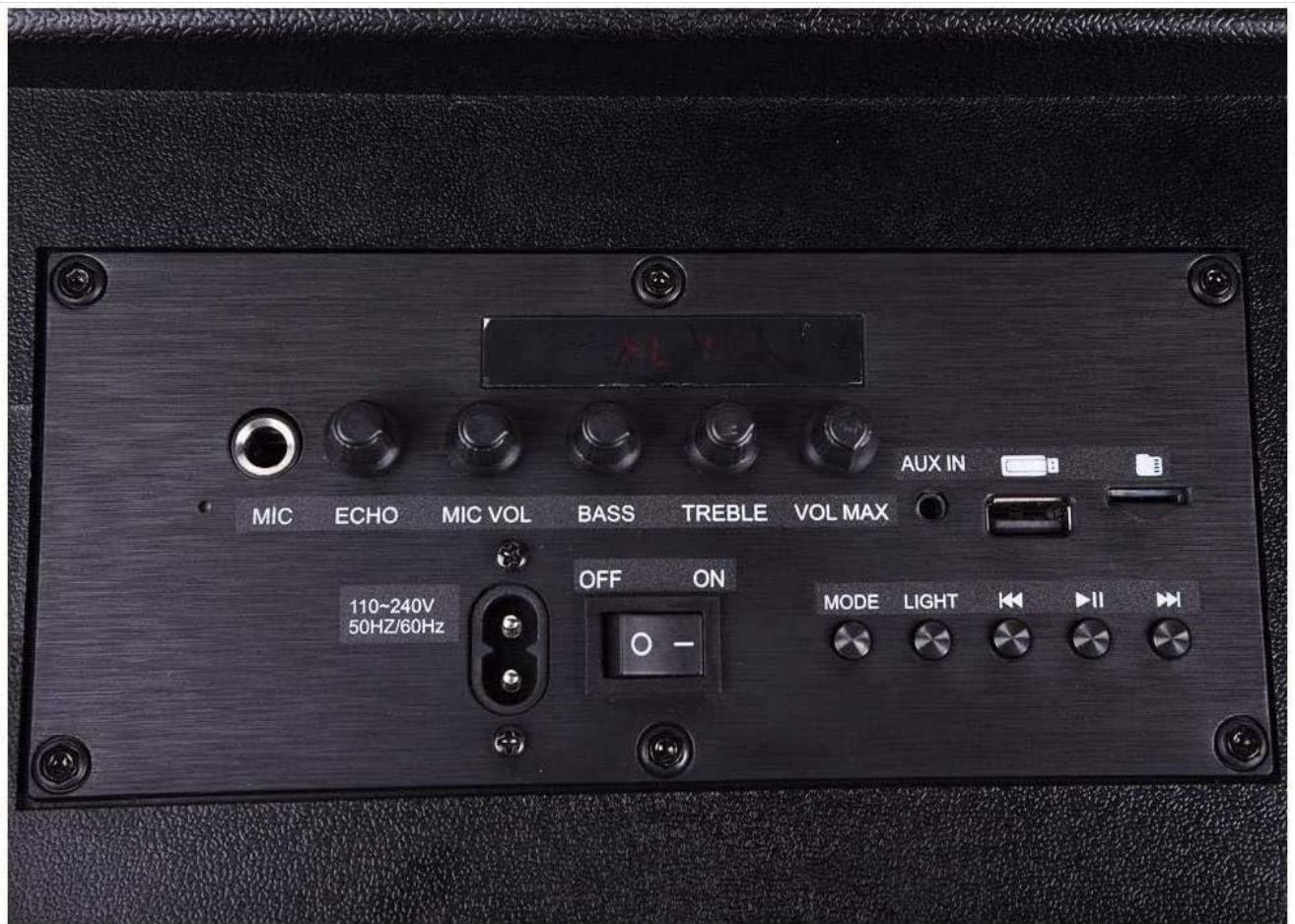
Figure 3: Detailed view of the control panel, showing inputs for MIC, AUX, USB, SD card, power switch, and various control knobs and buttons for audio adjustments and mode selection.
