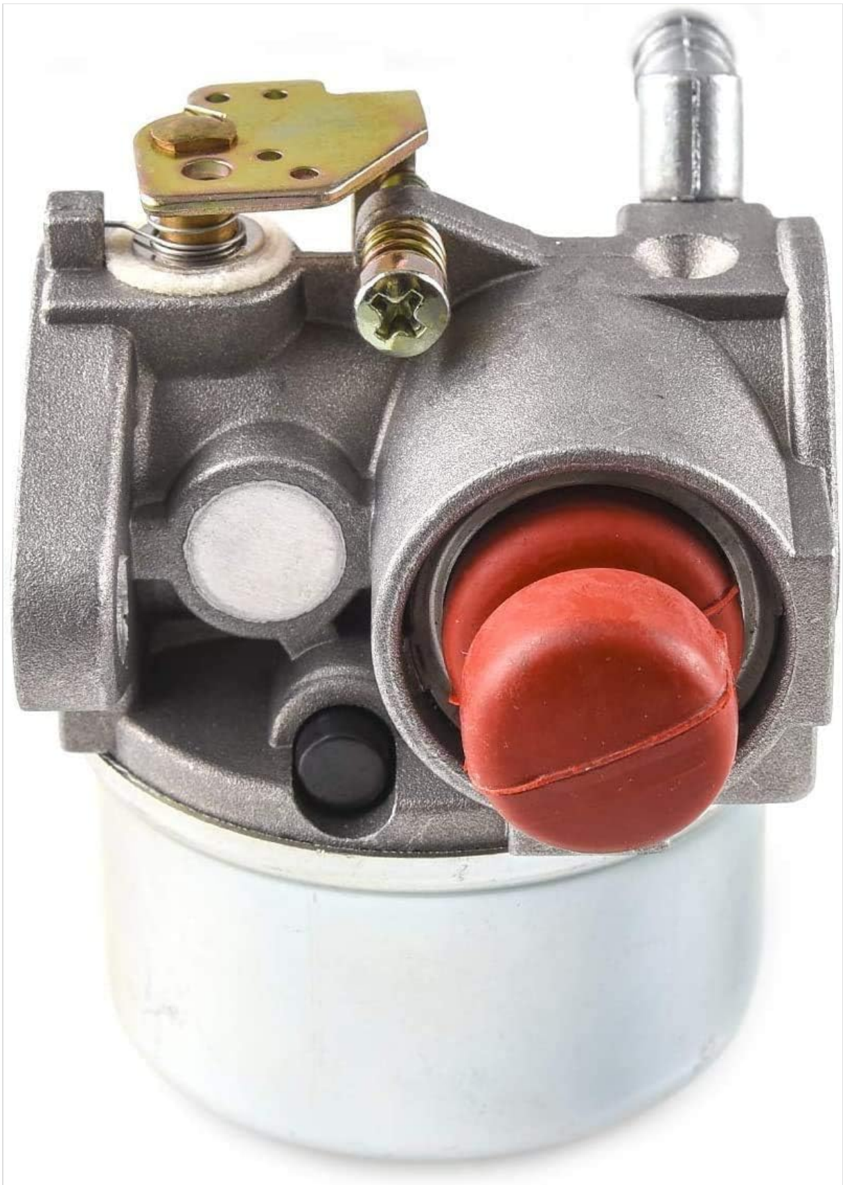
Figure 4: View highlighting the red primer bulb on the carburetor. The primer bulb is used to draw fuel into the carburetor for easier starting.
