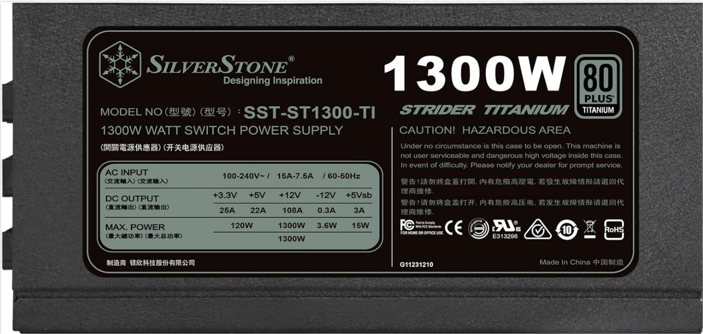
Figure 7: Top view showing the product specifications label.
